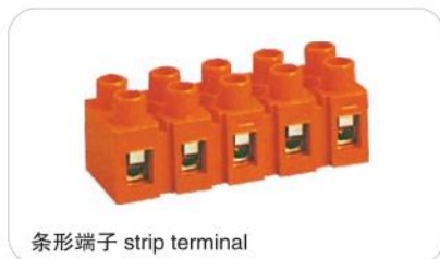
条形端子 strip terminal H 2519-5 导线截面 wire section: 0.5-6mm 2 额定电流/电压 rated current/voltage: 36A/600V 宽/高/厚 wide/high/thick: 50/21/21mm
