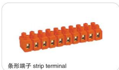
条形端子 strip terminal H 2519-10 导线截面 wire section: 0.5-6mm 2 额定电流/电压 rated current/voltage: 36A/600V 宽/高/厚 wide/high/thick: 122/21/21mm
