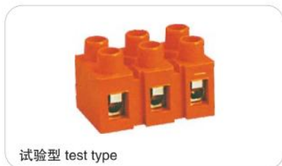
试验型 test type H 2519-3 导线截面 wire section: 0.5-6mm 2 额定电流/电压 rated current/voltage: 36A/600V 宽/高/厚 wide/high/thick: 33/21/21mm
