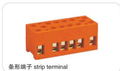
条形端子 strip terminal H 3801-6 导线截面 wire section: 0.5-6mm 2 额定电流/电压 rated current/voltage: 36A/600V 宽/高/厚 wide/high/thick: 53/21/21mm
